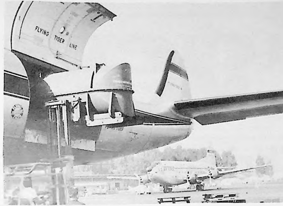
A jet engine goes aboard a Flying Tiger air freighter at a MATS base.
