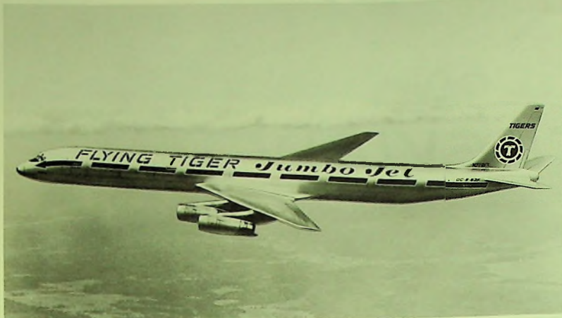
JUMBO JET ERA. First of the airlines to turn the corner into the jumbo jet era is the Flying Tiger Line. Beginning in late May 1968, the first of these huge DC8-63F airfreighters are expected to join the fleet. It will be the largest aircraft flying at that time, 37 feet longer than the conventional DC-8.
