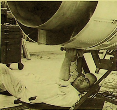
Lying down on the job: Carl Kenny checks the thrust reverser.
