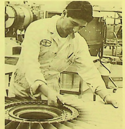
Jose Toro of Chile checks the security of the compressor disc fan blades.
