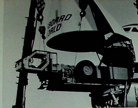
Outsized cargo is loaded with ease on board Seaboard's nose-loading B747. Flying Tigers' new B747-200s also have nose-loading capabilities.
