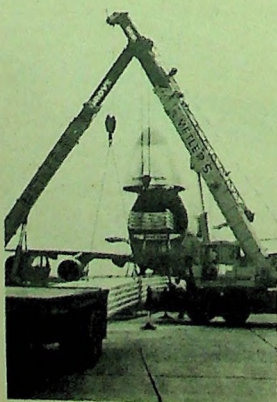
Off-loading in Knoxville — Huge and heavy bundles of ferris wheel spokes are off-loaded with the aid of cranes at McGhee-Tyson Airport in Knoxville. Two cranes were needed to compensate for the absence of 747 loading equipment at the airport.
