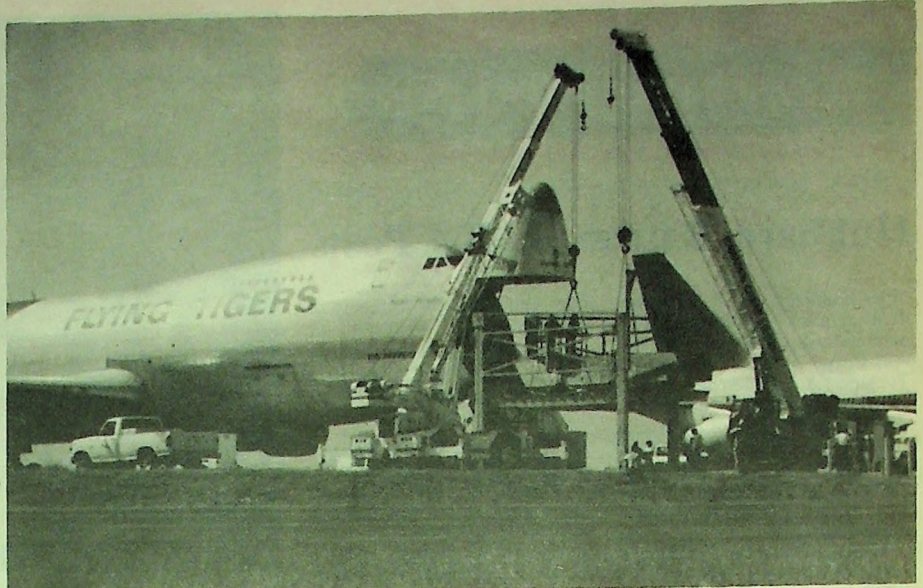
Two cranes are used to load 44,020-pound generator drive shaft in Honolulu for trip to Japan.
