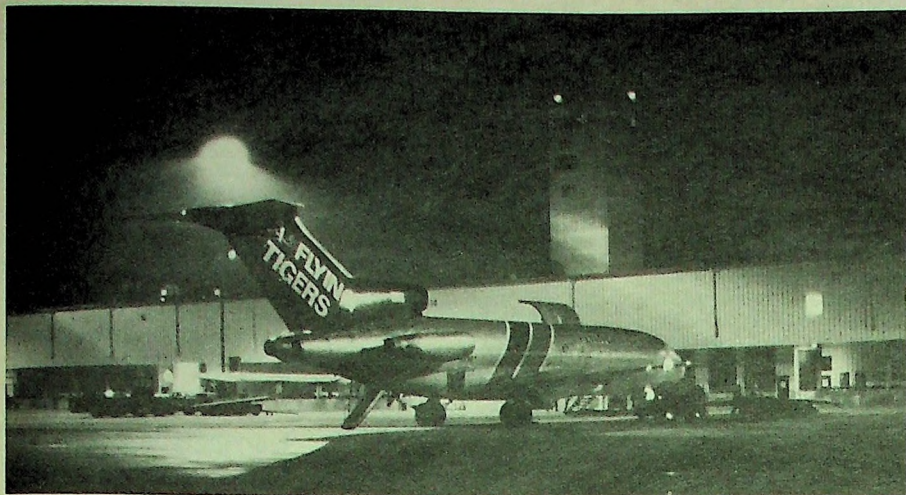
Above: B-727 jetfreighter at Flying Tigers' new Columbus hub building, showing the "crow's nest" observation tower where ramp operations can be observed and ground traffic controlled.
