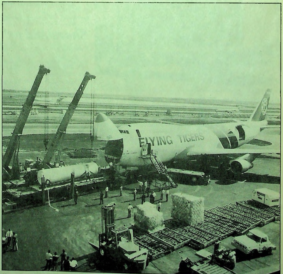
How to Feed a 747... A Flying Tigers' B-747 charter flight set a record for the airline in May when it carried a 97,000 pound chemical compressor reactor from Chicago to Brussels, Belgium—marking the heaviest single shipment ever carried by Flying Tigers. Two 60-ton cranes were utilized to onload the reactor, which is 38-feet long, 8-feet in diameter and 2-inches thick. One of only five reactors of its kind in the world, the unit, shown above as it was about to be loaded into the nose of the aircraft, will be used to produce plastics and polystyrene products.
